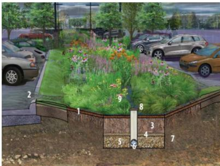
Image 2: Rendering of a typical bioretention area. (Image source: Johnson County Soil and Water District)
