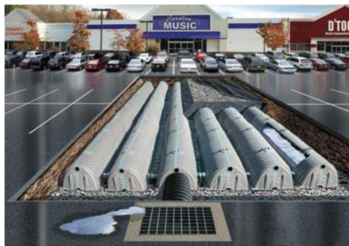
Image 3: View of typical underground infiltration system beneath a parking lot. (Image source: www.kitchener.ca)
